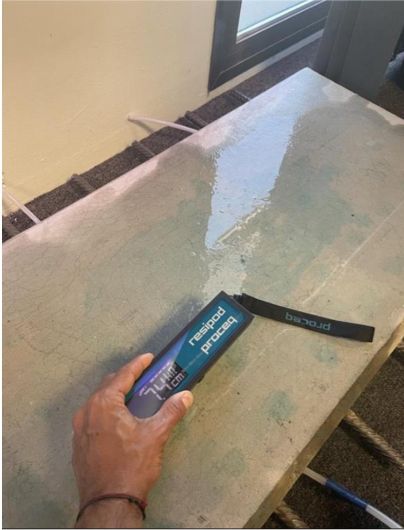
Concrete resistivity results using Resipod
