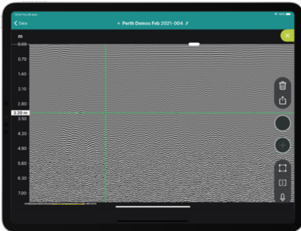
Small target detected at more than 3.2m depth (refer to the intersection of the green cursors).
