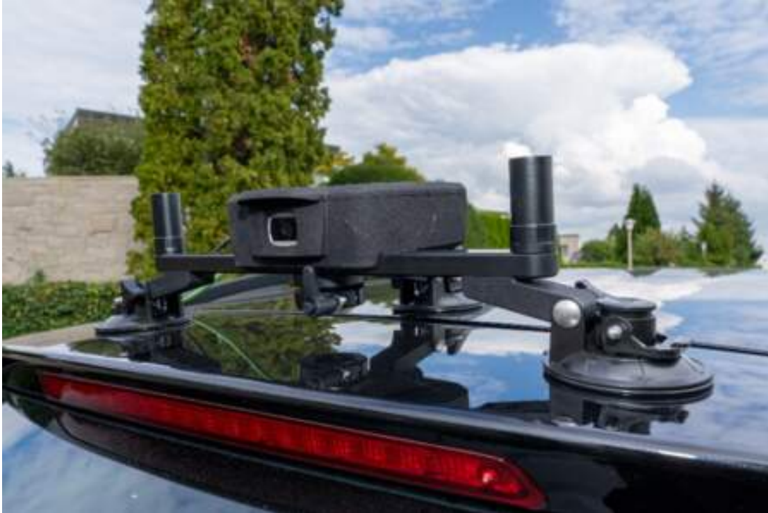
Figure 5. Visual odometry-based system for data positioning.
