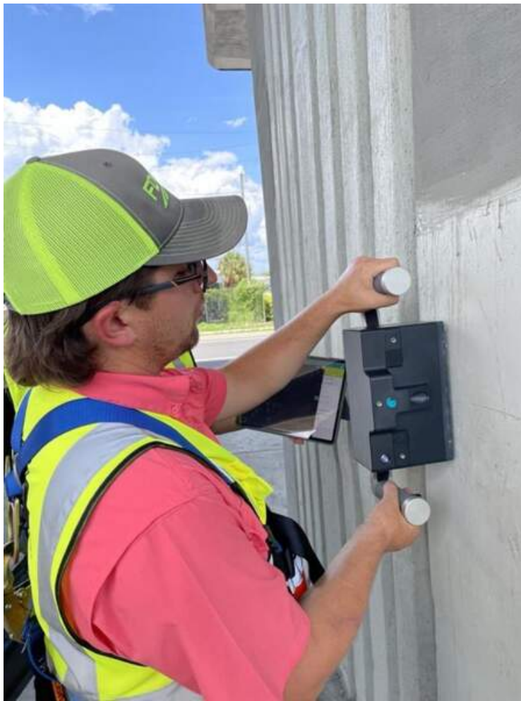
The Pundit PD8050 ultrasonic pulse echo system
