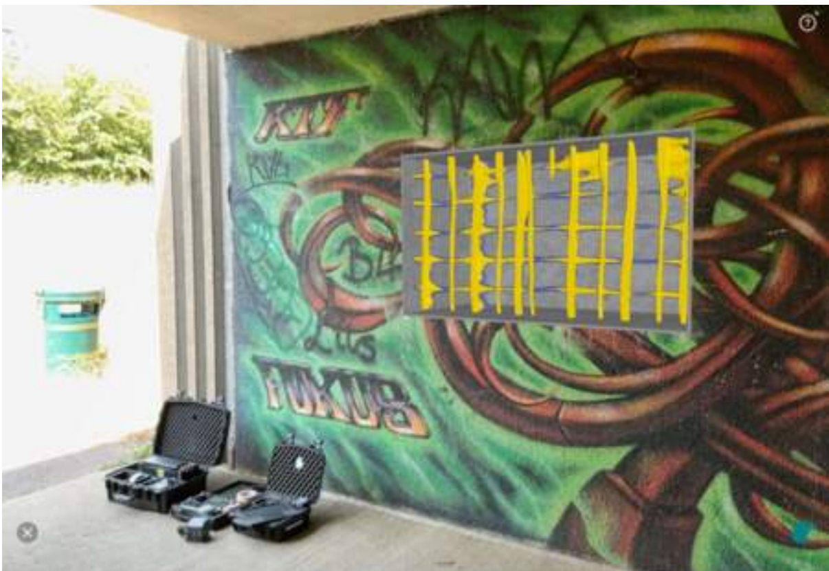
GPR data in 3D augmented reality projections with the GP app
