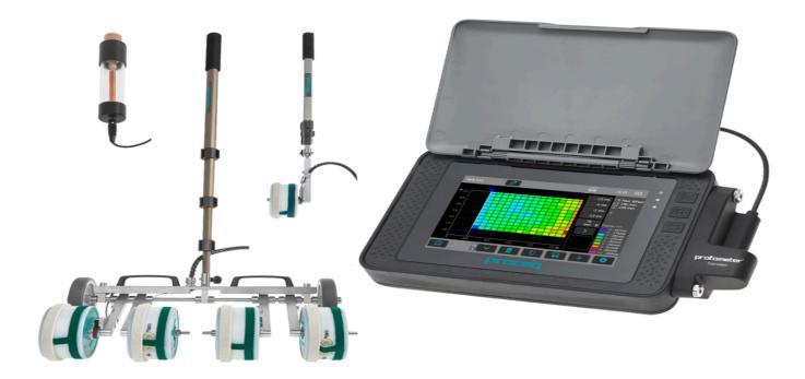
Half-cell Corrosion Potential
