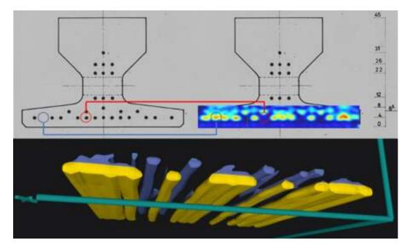
Two examples of this are shown in the image – the blue circle shows a location where there was thought to be no prestressed reinforcement strands but actually they were present, and the red circle shows a location where the converse was true. Therefore the GPR inspection prevented structural elements from being damaged when cores were removed for laboratory assessment.
