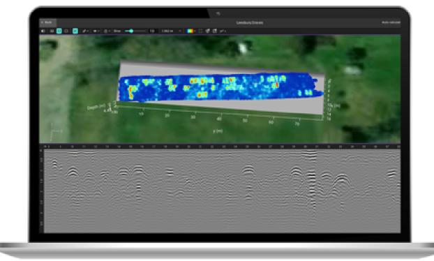
GPR data visualized using post-processing software, GPR Insights
