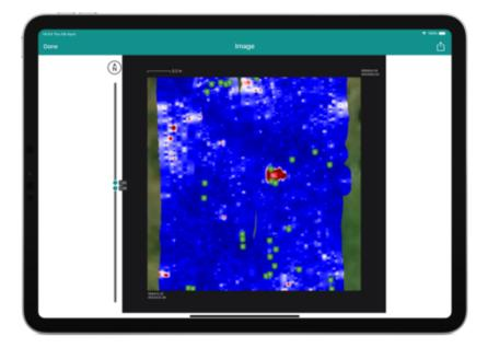
All inspection data is automatically synchronized to the cloud and the Screening Eagle Workspace platform. From there, the team are able to easily access the data and perform post-processing using <u>GPR SLICE and</u> <u>GPR Insights</u>.
