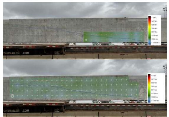
It was clear from the results that the velocities were similar throughout the measurement grid and do not indicate discrepancies or areas of weakness. Therefore, the UPV measurements indicated the beam has been placed monolithically and did not suggest the presence of a cold joint or discontinuity.
