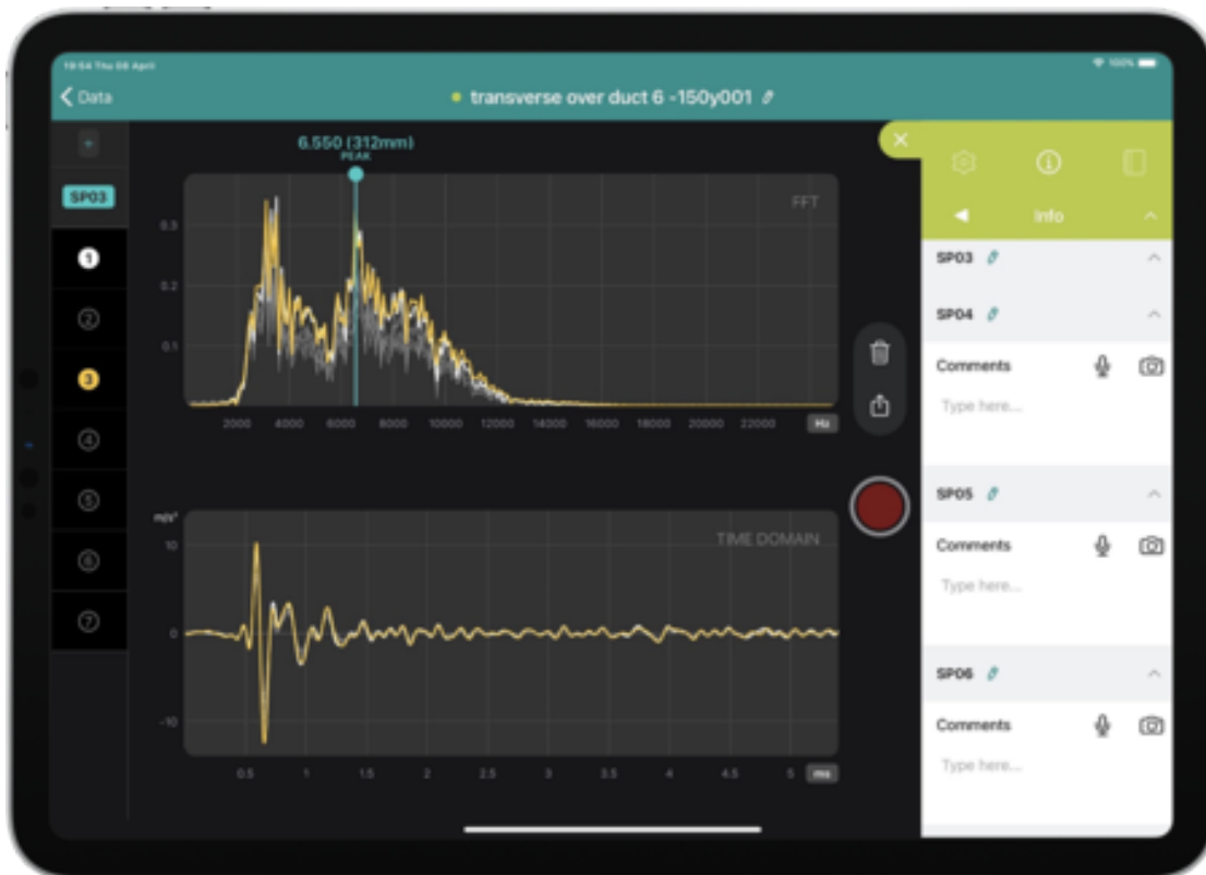
Air voiding as shown with Pundit PI8000 ultrasonic impact echo technology, taken in the same spot as the PD8050.
