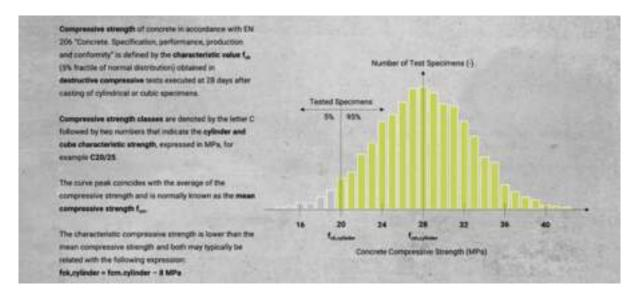
It is true, traditional methods of concrete strength testing is not that straight-forward and is pretty costly. Furthermore, concrete is never uniform. If you take samples while pouring concrete, these samples are not placed, compacted or cured like the concrete placed in the real structure. Meanwhile core samples from an existing structure are disturbed during the extraction process. All these factors affect the estimated strength value.
