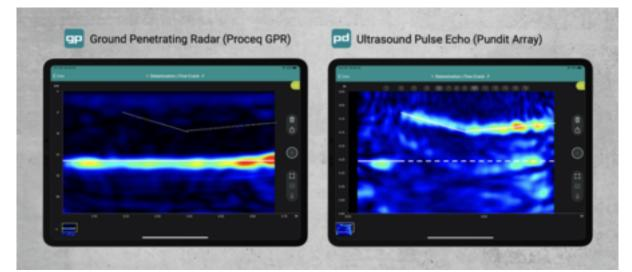
As you know, GPR is perfect for detecting metal objects like rebar. When the GPR waves hit metal, they reflect 100% and you get a very strong signal back. Although GPR provides accurate data for most concrete evaluations, there are some instances where it can have limitations:
