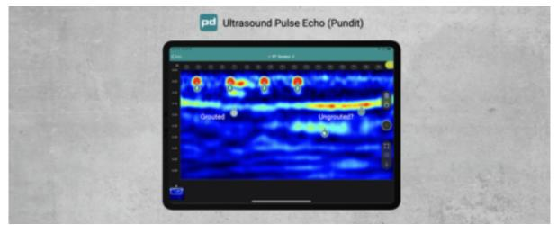
Evaluate the homogeneity and the quality of the concrete, detect internal defects, and estimate the depth of any cracks using ultrasonic tomography with the Pundit Live Array.
