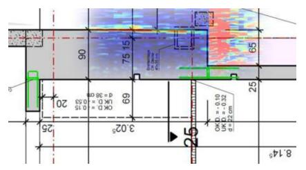
Screening Eagle Technology's portable ultrasonic imaging device, <u>Pundit PD8000</u>, is used to generate 2D and 3D images of concrete structures up to 2m thick. The images are generated immediately on site. The high signal-to-noise ratio and advanced imaging algorithms produce high quality images from which defects can be quickly identified and tagged. Views and maps are also instantly available in the field.
