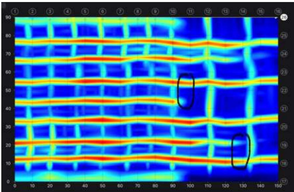
The information collected with the [GP8000](#) is incorporated into a calculation model, so that the force effect of the bridge can be determined.
