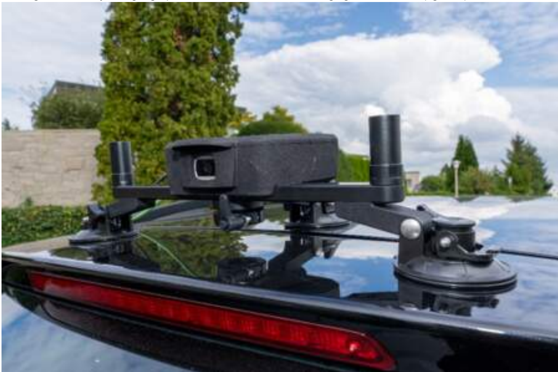
Figure 5. Visual odometry-based system for data positioning.
