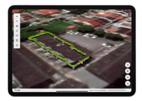
An area scan of 7m by 3.5m with a spacing of 0.25m was performed and the pipe was located. The team were able to see the pipe, its direction and depth and visualize it in Augmented Reality, enabling them to understand its exact location.
