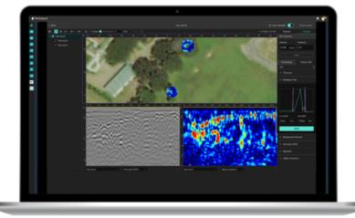
Since the GS8000 data was collected with centimeter level accuracy GNSS, depth-slice results could be superimposed on a satellite map. We can easily understand the distribution of tree root system within the measurement coverage. By pinpointing (e.g., double click) on any position we can locate how the tree root architecture looks like at actual depth.
