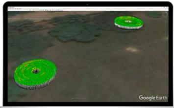
GNSS positions around the two trees, overlaid on Google Earth image. Green colour indicates an excellent GNSS correction status and yellow indicates a less good status.
