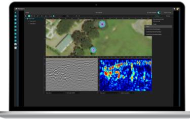
With its automatic processing and cloud computing power, 2D radargram and 3D slice view were automatically generated in less than a few minutes.
