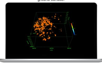
3D results displayed in GPR-SLICE. The 3D orange shapes are areas of higher reflection amplitude and they represent the architectures of tree roots, in particular the anchorage roots.
