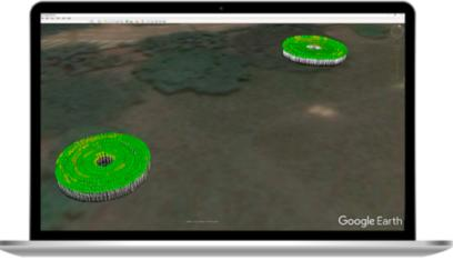
GNSS positions around the two trees, overlaid on Google Earth image. Green colour indicates an excellent GNSS correction status and yellow indicates a less good status.
