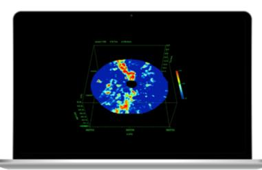
2D results of one tree displayed in GPR SLICE. A depth or time-slice view is shown. This is a cross-section parallel to the ground surface.
