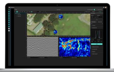
Since the GS8000 data was collected with centimeter level accuracy GNSS, depth-slice results could be superimposed on a satellite map. We can easily understand the distribution of tree root system within the measurement coverage. By pinpointing (e.g., double click) on any position we can locate how the tree root architecture looks like at actual depth.
