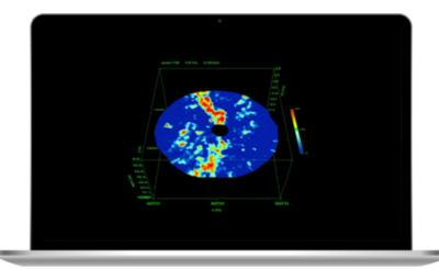
2D results of one tree displayed in GPR SLICE. A depth or time-slice view is shown. This is a cross-section parallel to the ground surface.
