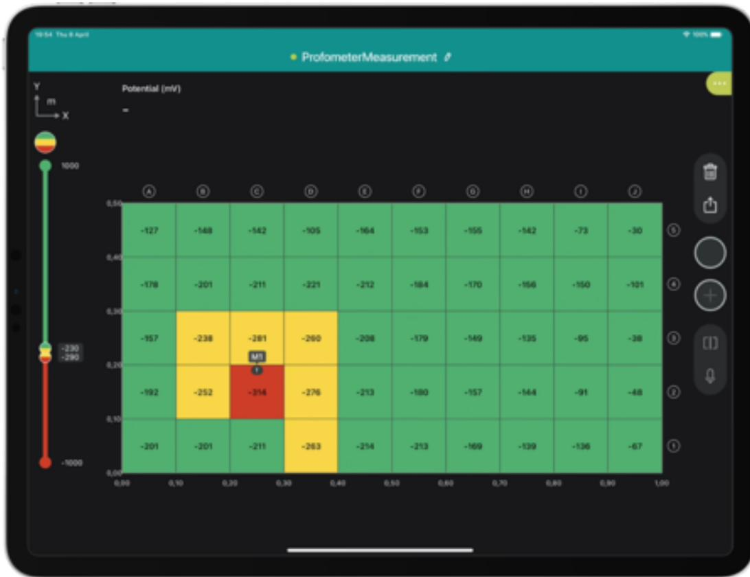
Corrosion likelihood using Profometer PM8500 Corrosion
