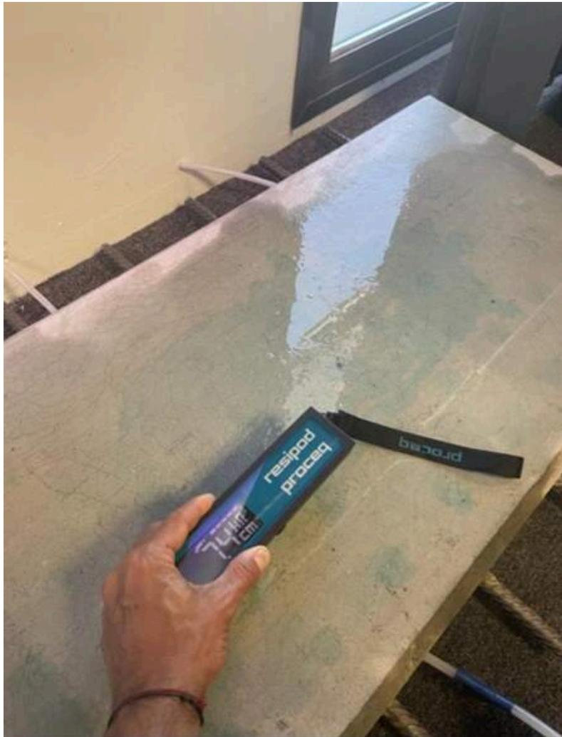
Concrete resistivity results using Resipod
