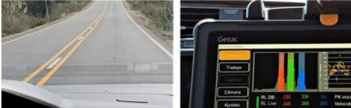
Example of a road with triple road markings (left) and the results as seen live on ZDR6020 software (right).
