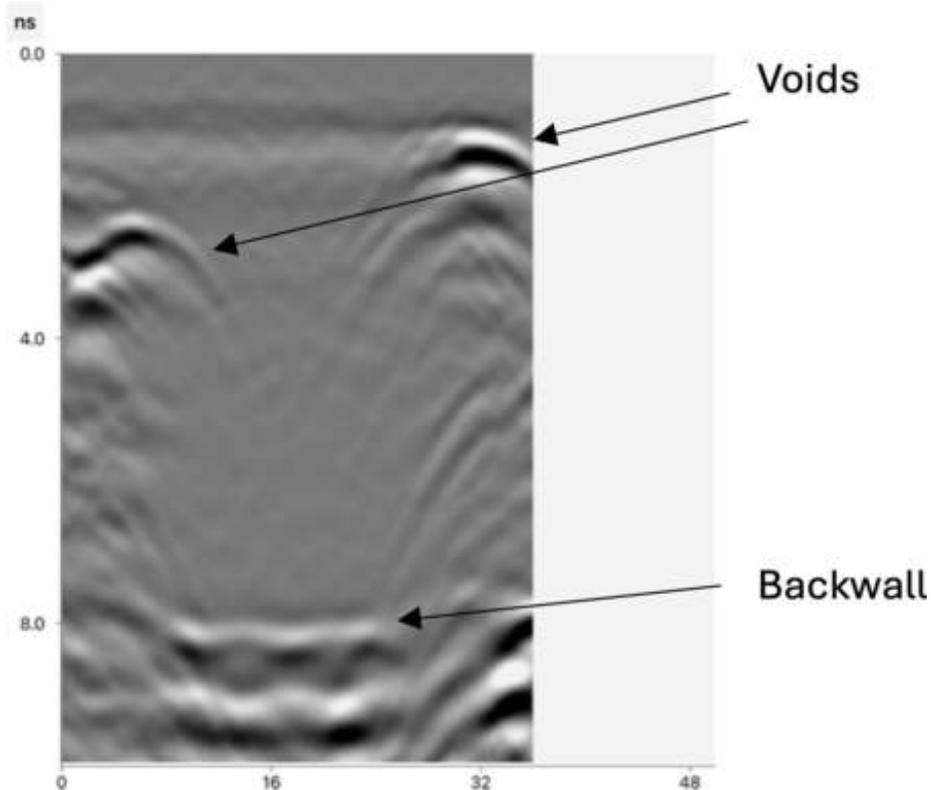
Figure 2: GPR scan showing air in concrete
