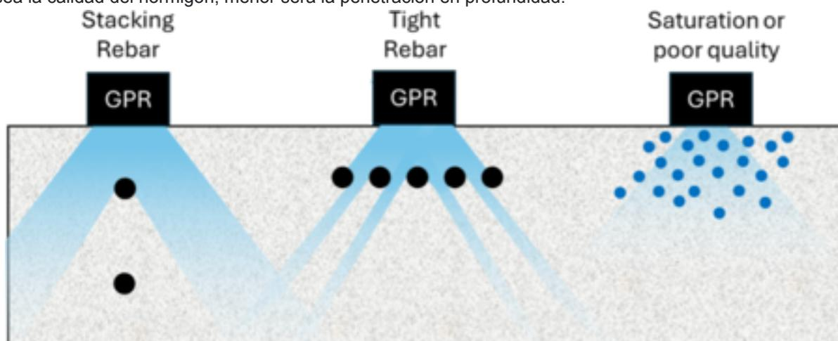
Figure 3: Factors limiting GPR imaging
