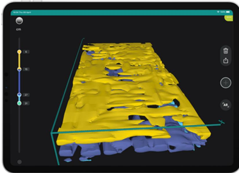
3D view of the top shift (yellow line) and mortar joint between second stone shift (dark blue line)
