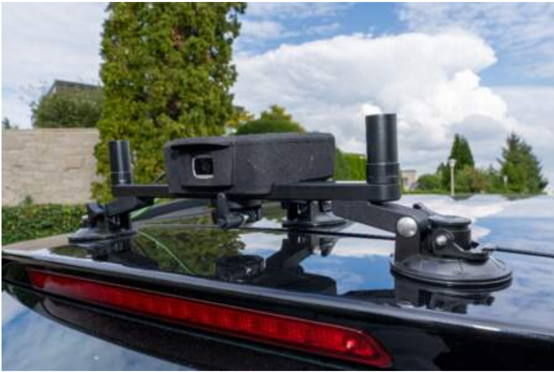
Figure 5. Visual odometry-based system for data positioning.
