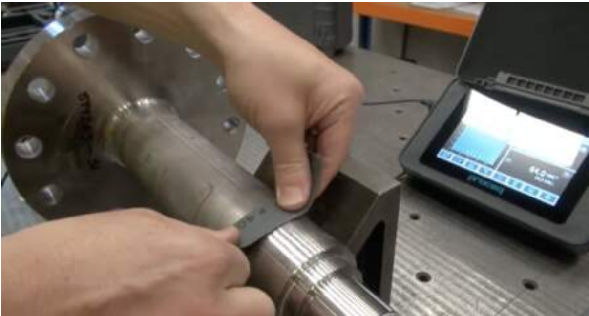
Fig. 5 — preparing the surface with sandpaper
