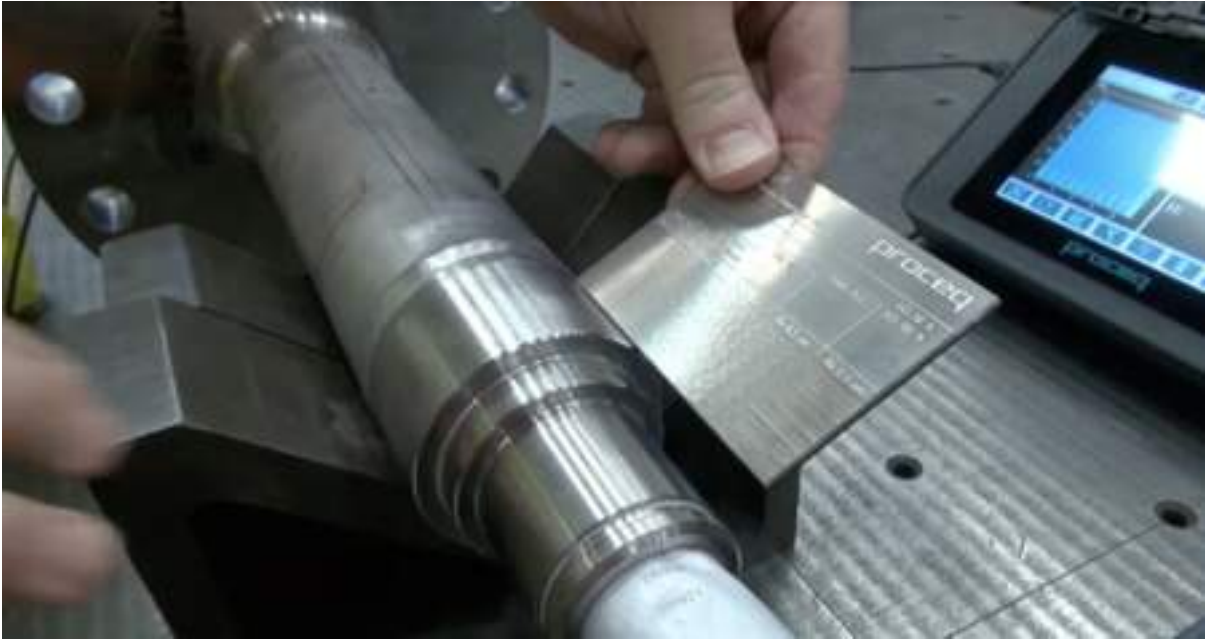
Fig. 6 — Checking the surface roughness comparator plate again
