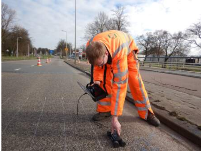
Using the Profometer on the bridge
