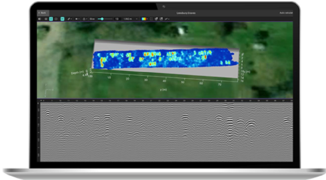
GPR data visualized using post-processing software, GPR Insights
