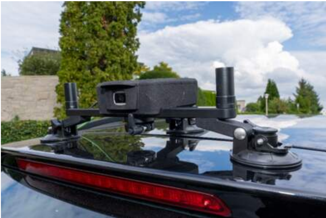
Figure 5. Visual odometry-based system for data positioning.
