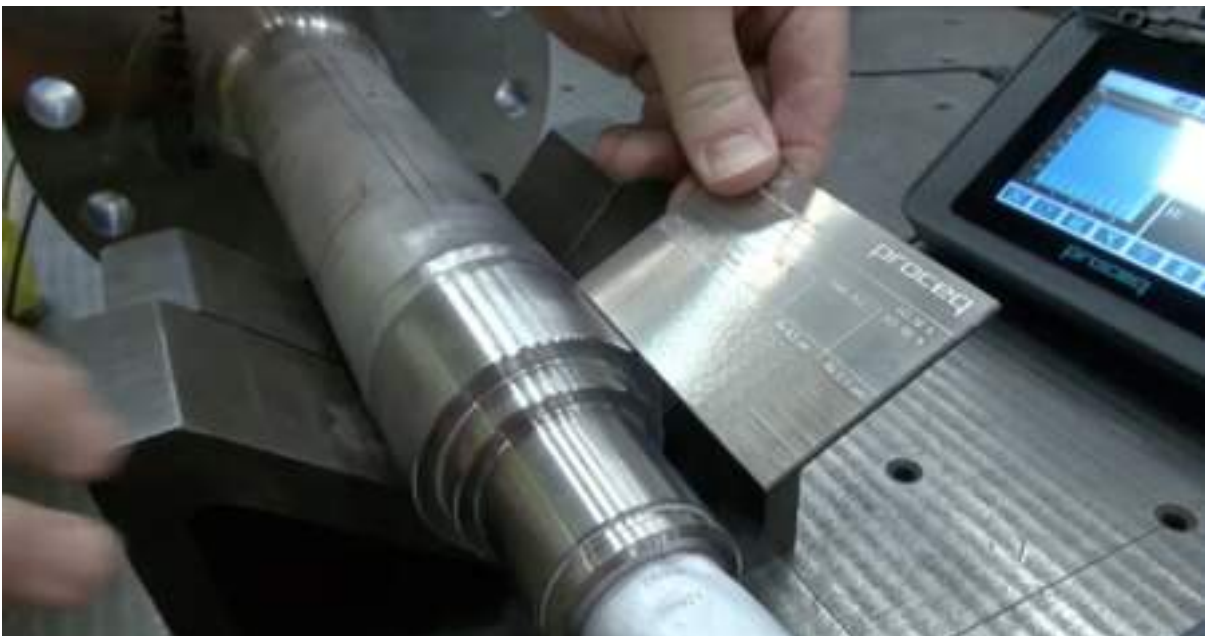
Fig. 6 — Checking the surface roughness comparator plate again
