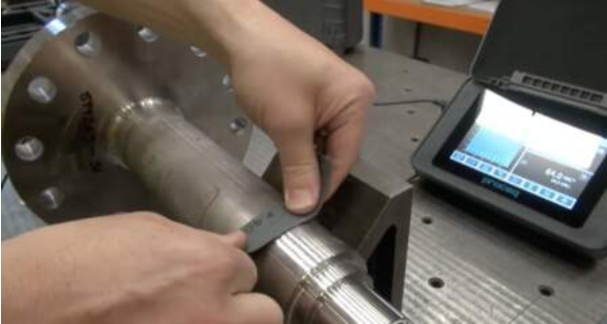
Fig. 5 — preparing the surface with sandpaper
