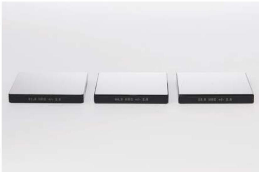
Equotip Portable Rockwell Test blocks
