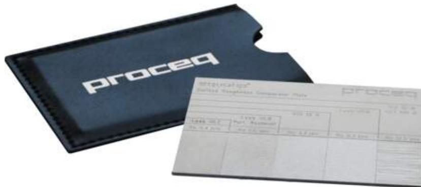
Equotip Surface Roughness Comparator
