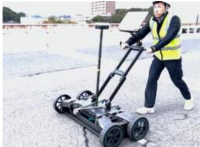
Figure 2 and Figure 3 show the GS9000 system operating on the bridge deck
