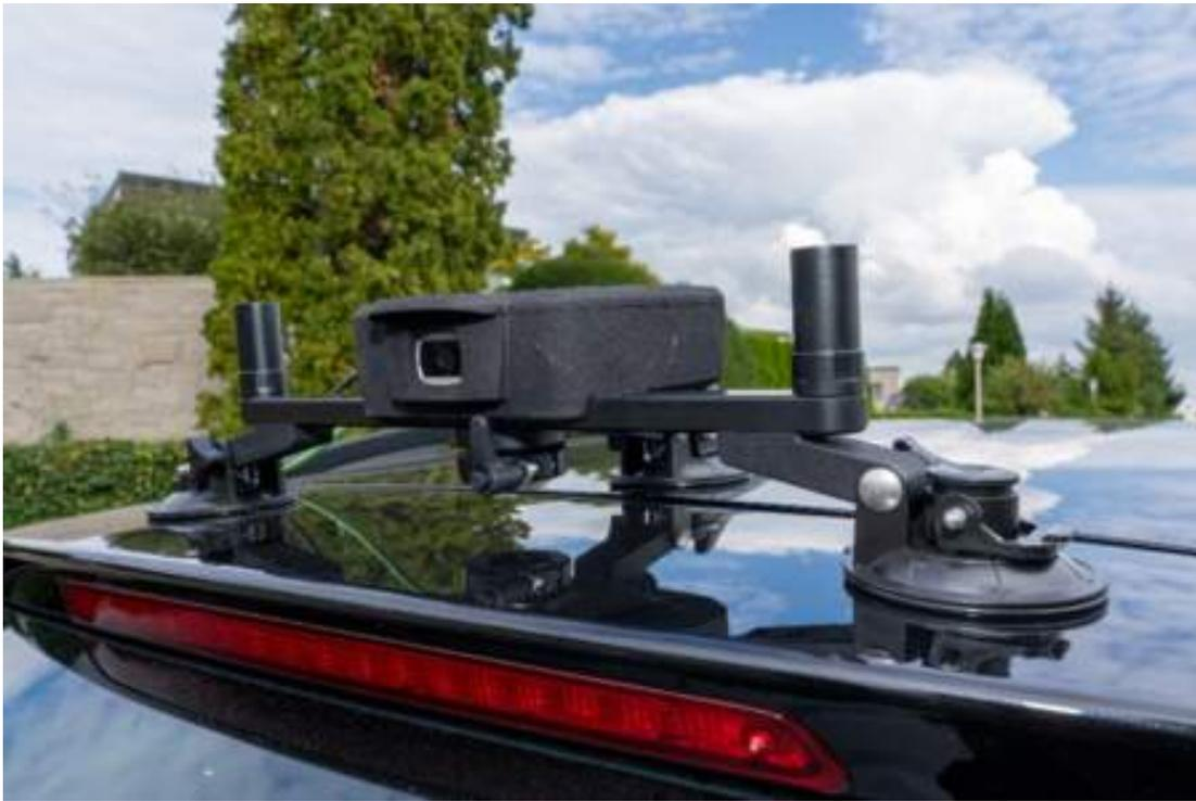
Figure 5. Visual odometry-based system for data positioning.
