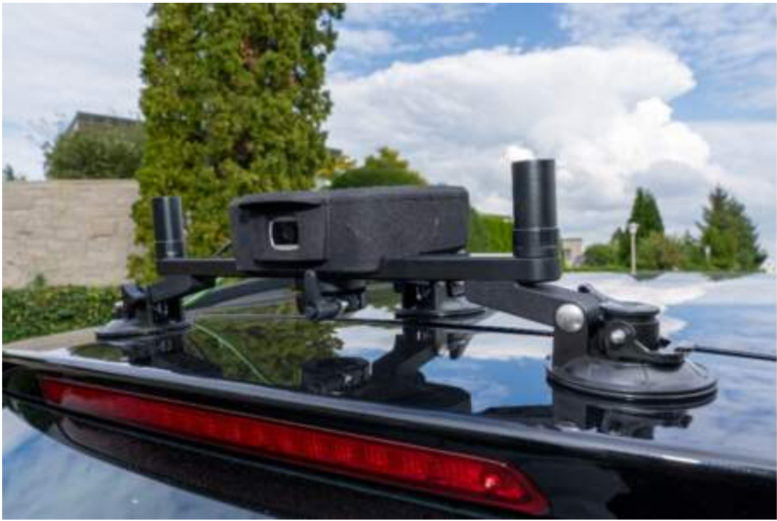
Figure 5. Visual odometry-based system for data positioning.
