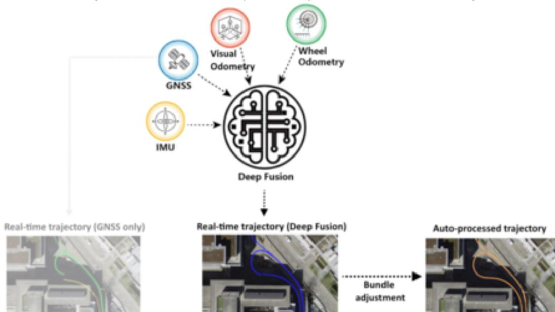
Figure 6. Advanced sensor fusion for accurate trajectory calculation
