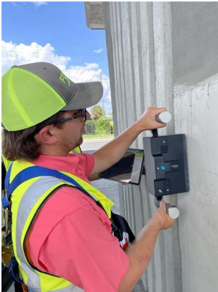
The Pundit PD8050 ultrasonic pulse echo system
