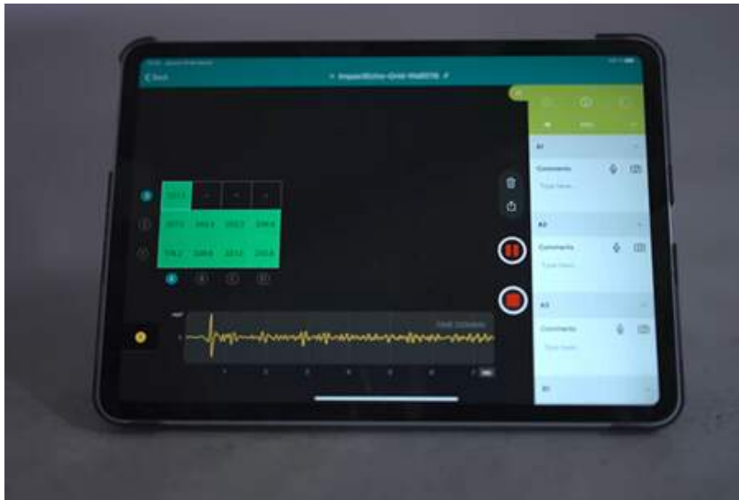
Impact Echo grid mode on the PI8000 app
