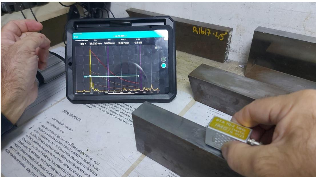
After the calibration the 2nd level has performed the inspection sharing video, in real-time.
