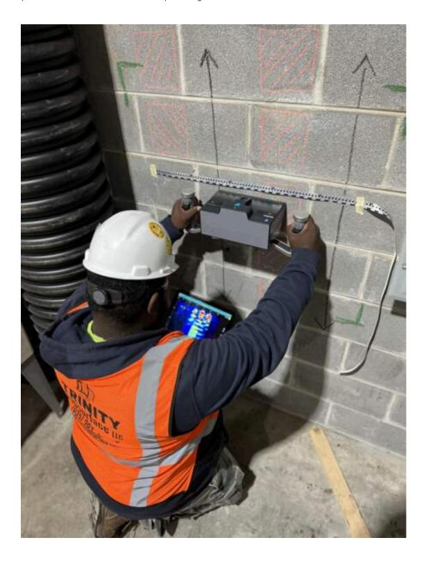
For large areas of different shapes, the team make good use of the Proceq GS8000 Pro's 'free path' feature which allows them to scan the subsurface as they walk freely, unconstrained by a grid.
