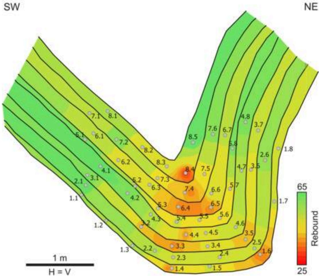
Figure 1: Geological profile across the studied syncline including contours of equal Schmidt hammer rebound constructed using data from 55 stations. Each station has been labelled with two numbers separated with a dot. The first number is the bed number, whereas the second number is the station number.
