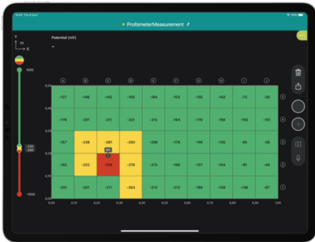
Corrosion likelihood using Profometer PM8500 Corrosion
