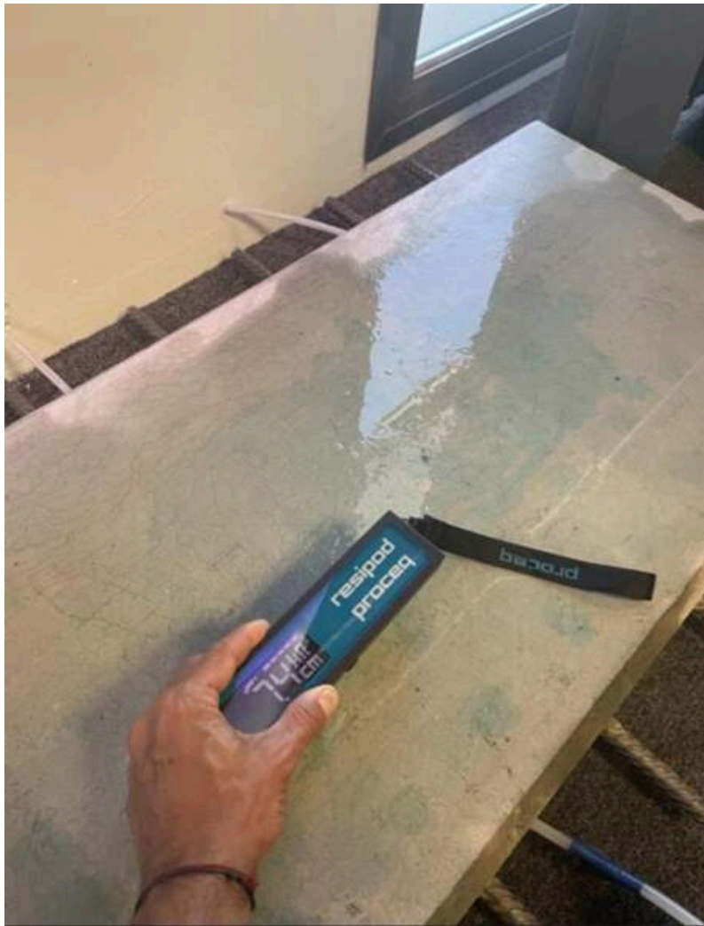
Concrete resistivity results using Resipod
