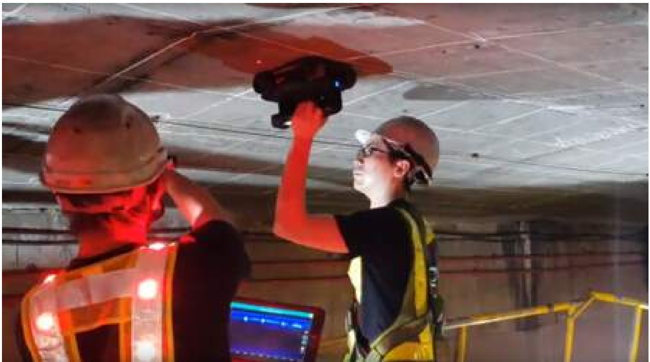
The Proceq GP8000 GPR scanning thick concrete
