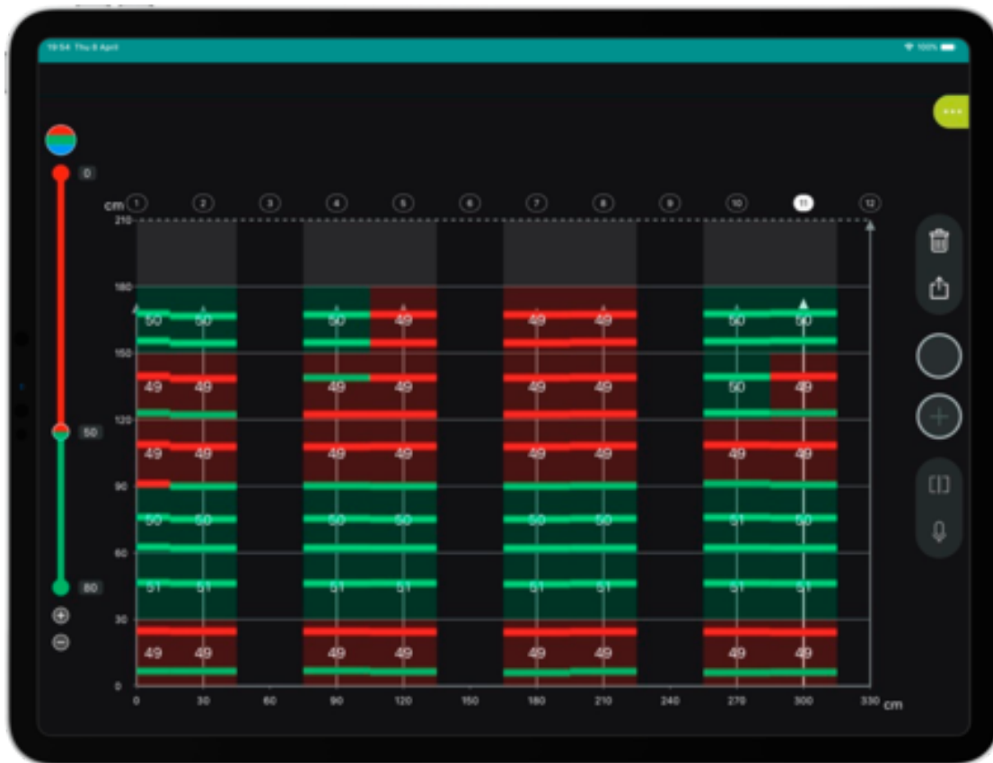
Scanning column's stirrups in vertical scanning direction
