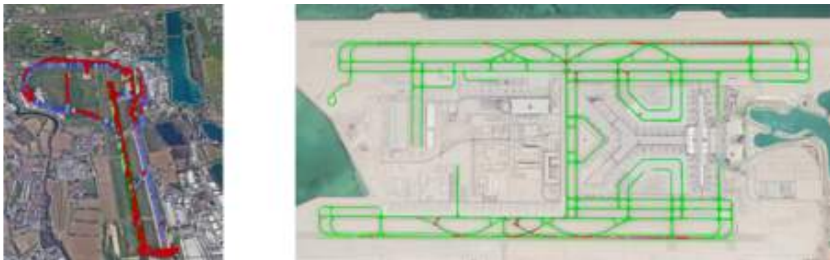
ZDR6020 Retroreflection results from airports in Europe (left) and Middle East (right) superimposed on maps. The green/red/blue colours indicate different retroreflectivity ranges.
