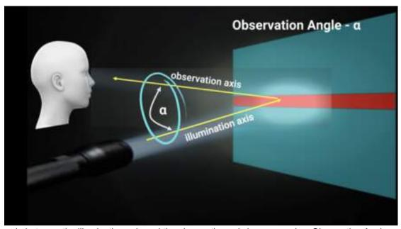
The angle between the illumination axis and the observation axis is measured as Observation Angle – a.
