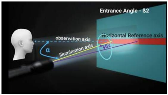
An Entrance Angle ( $\beta$ ) that is too large (i.e., the light hits the tape at a very sharp, oblique angle), the retroreflective elements become less effective.
