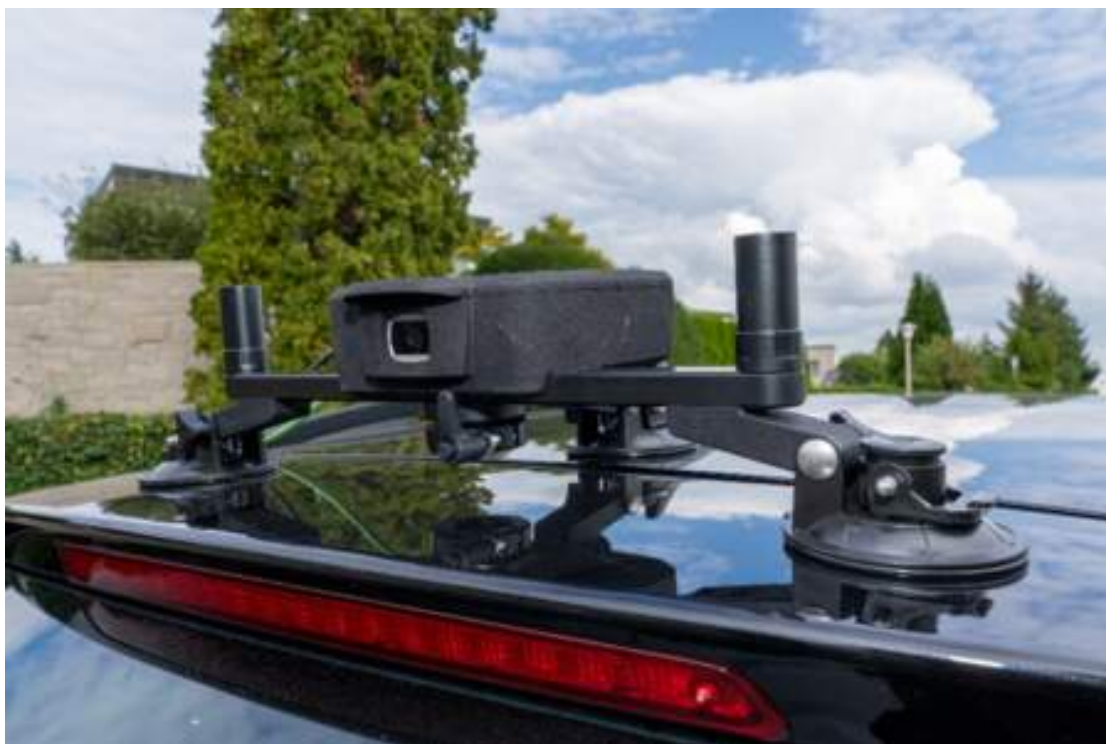
Figure 5. Visual odometry-based system for data positioning.
