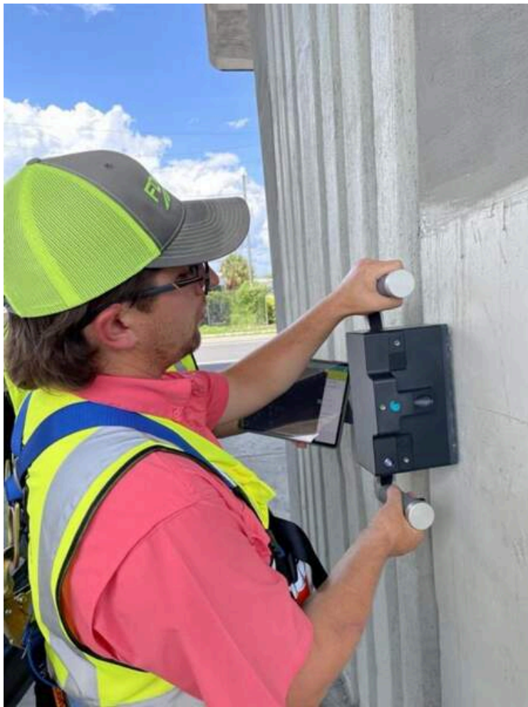
The Pundit PD8050 ultrasonic pulse echo system
