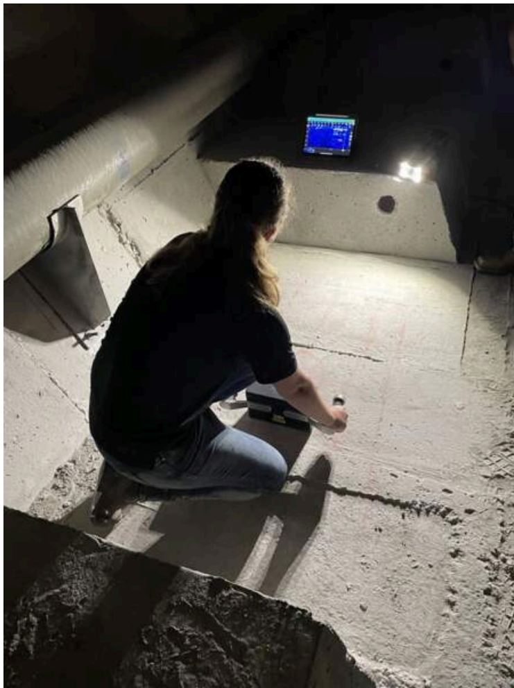
The Pundit PD8050 ultrasonic pulse echo system
