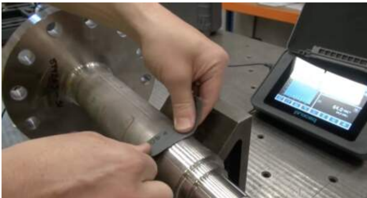
Fig. 5 — preparing the surface with sandpaper
