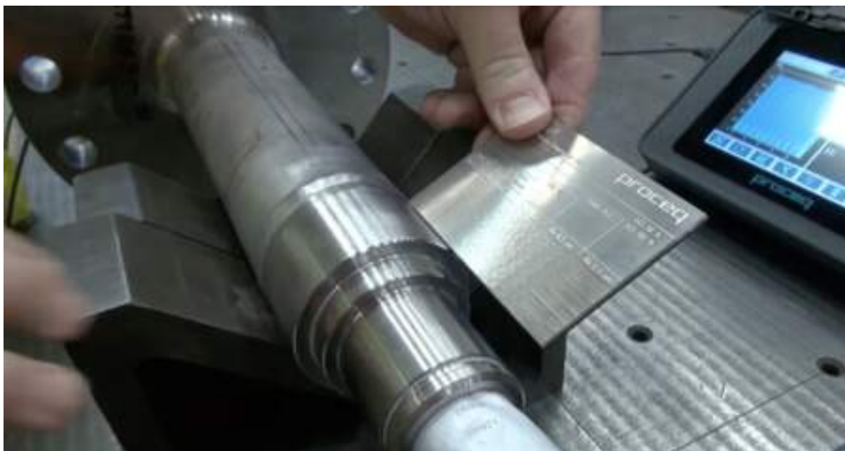
Fig. 6 — Checking the surface roughness comparator plate again
