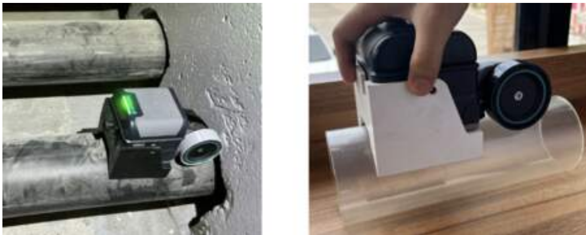
Figure 4: Saddle positioning in the field
