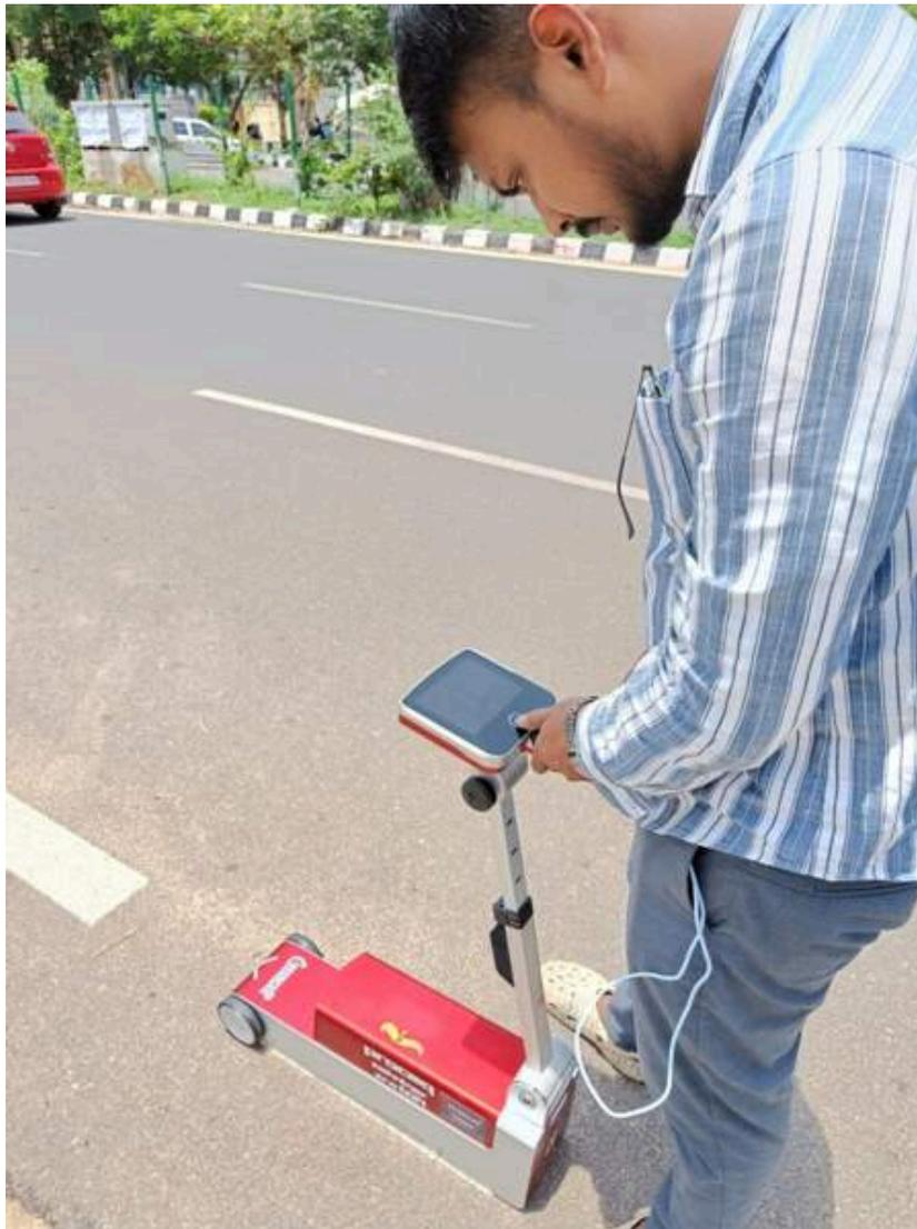
Enabled with 5.7" high-resolution color touchscreen, the retroreflector offers excellent visibility under all light conditions. The retroreflector logs all measurements with precise geolocation & provides comprehensive reports quickly with the help of user-friendly reporting software at ease.
