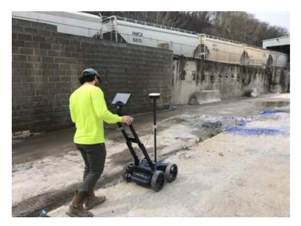
The team at YSU are working to improve the success rate of the geophysical survey (including GPR) through a better understanding of the long-term and seasonal relationship between organic decomposition and resulting geophysical signatures. They have set up an extensive test site to do this using pig carcasses, which have similar masses and body compositions to humans. The pigs are buried in different geological conditions e.g. dry, wet, with roots present etc.
