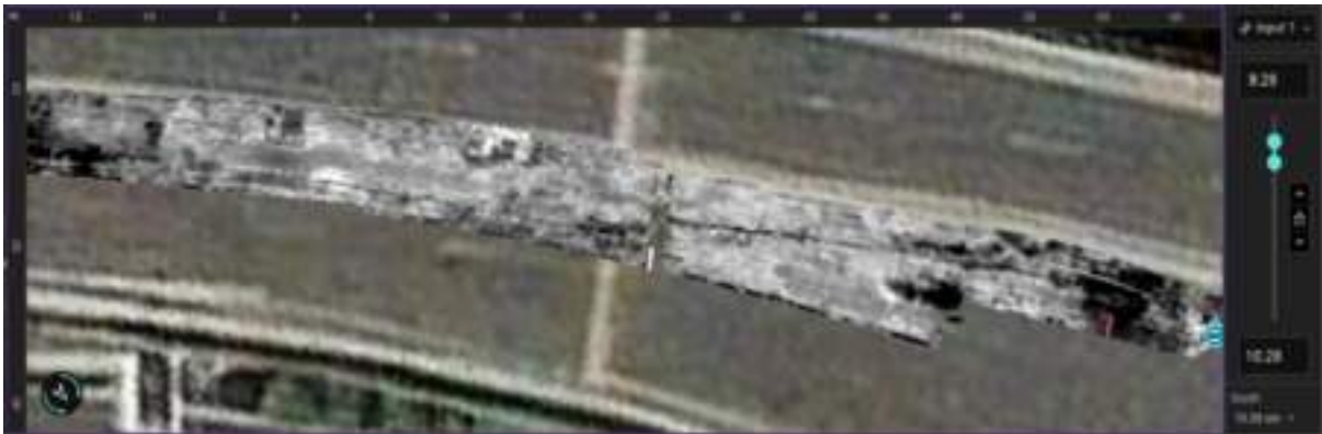
Figure 7. Interface defects between Asphalt-to-Concrete (A/C) layers (Delamination.)
