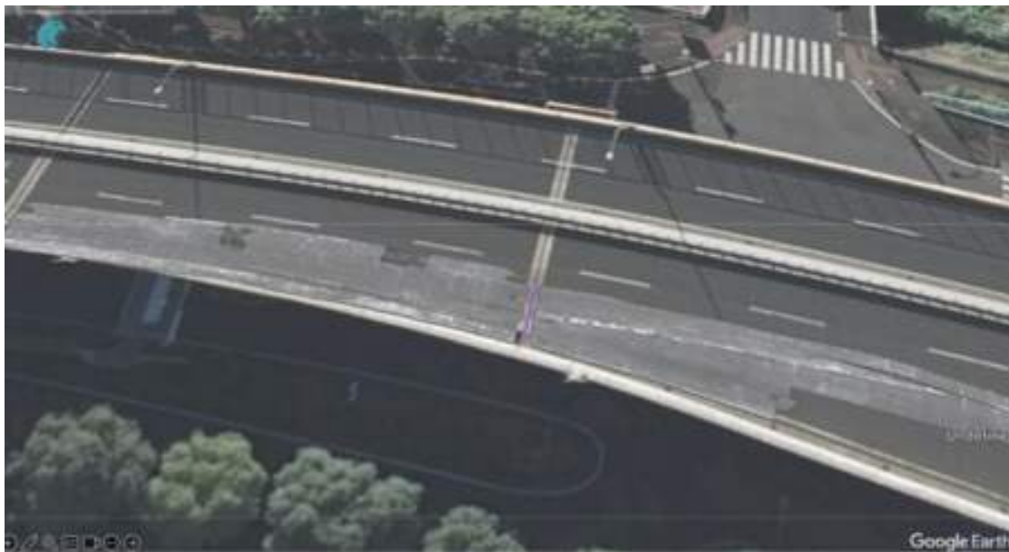
Figure 1. C-scan view overlaid in Google Earth, depicting the analysis of surface defects obtained from GPR Insights data collected by the GS9000.
