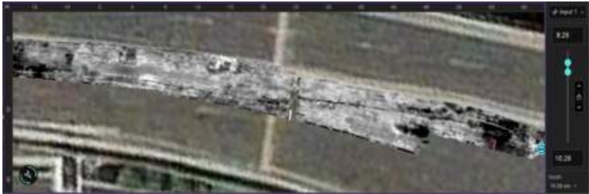
Figure 7. Interface defects between Asphalt-to-Concrete (A/C) layers (Delamination.)
