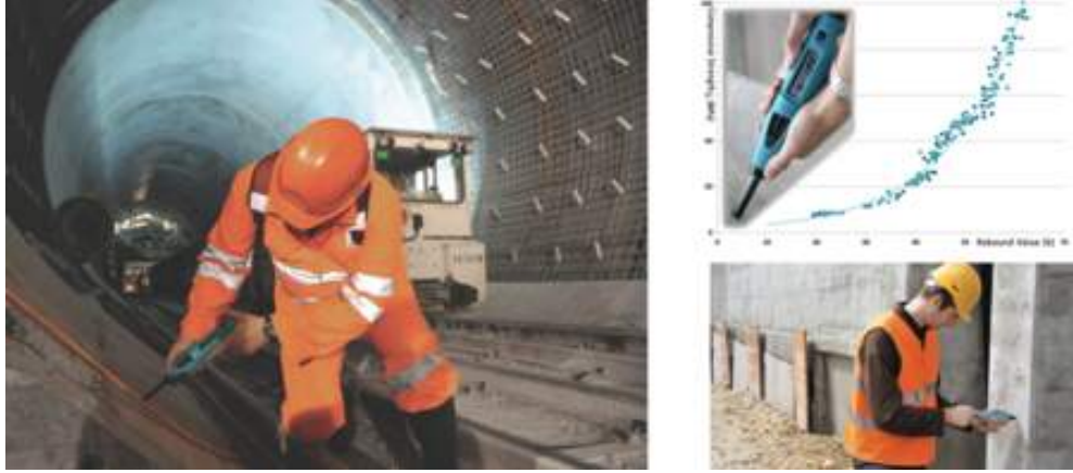
Next generation rebound hammer for concrete, the Silver Schmidt
