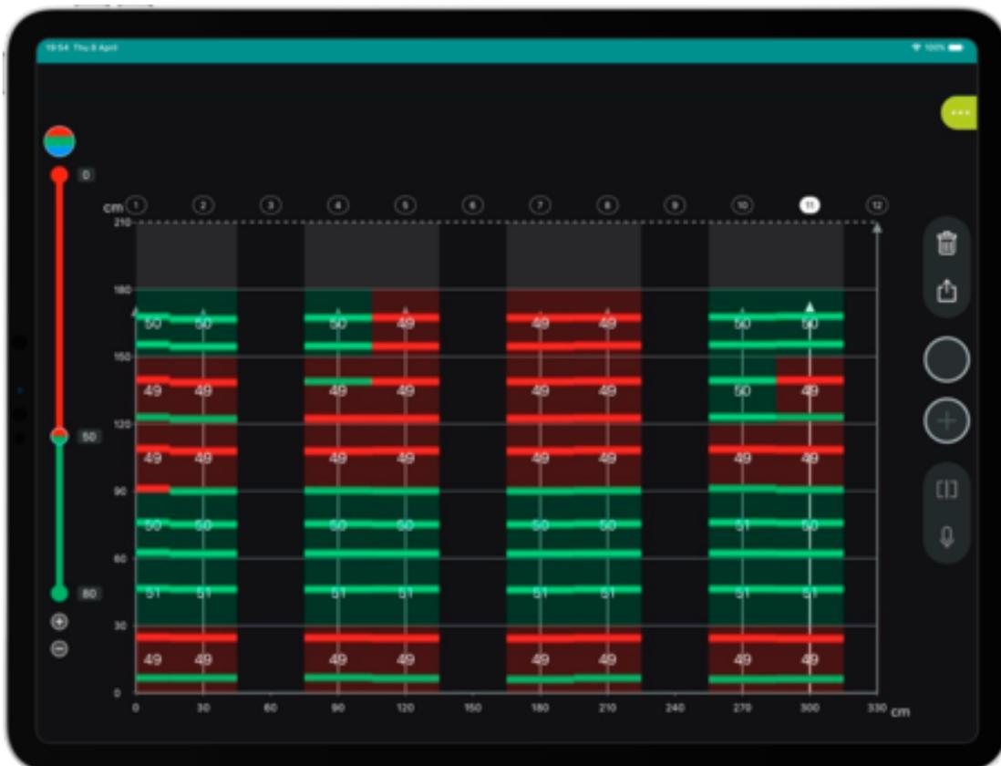
Scanning column's stirrups in vertical scanning direction
