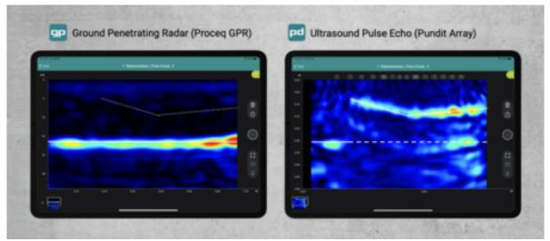
As you know, GPR is perfect for detecting metal objects like rebar. When the GPR waves hit metal, they reflect 100% and you get a very strong signal back. Although GPR provides accurate data for most concrete evaluations, there are some instances where it can have limitations:
